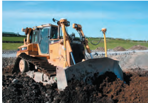
All of Maveric Constructors' equipment is outfitted with Trimble hardware and is managed via Trimble Construction Manager software.
